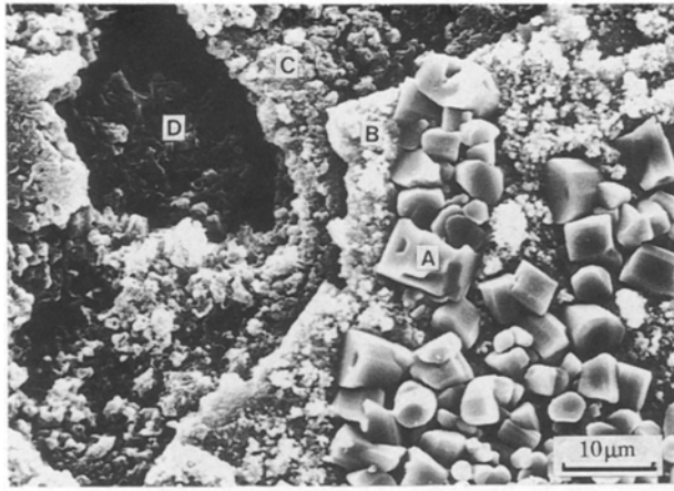
Figure 6 The reaction layers revealed after removing the brazing alloy by deep etching of the brazement by the Cu-5 at % Ti alloy at 1100 °C for 3600 s.
